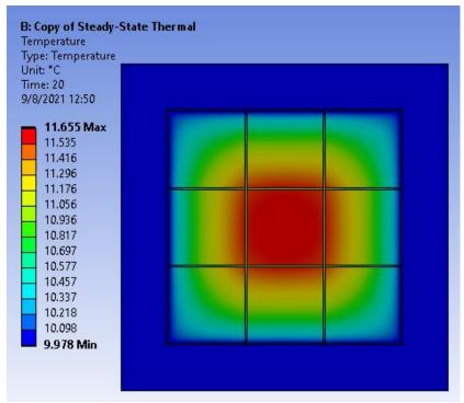
Rear face with 0.5 W heat load applied to each crystal; copper shell held at constant 10°C
